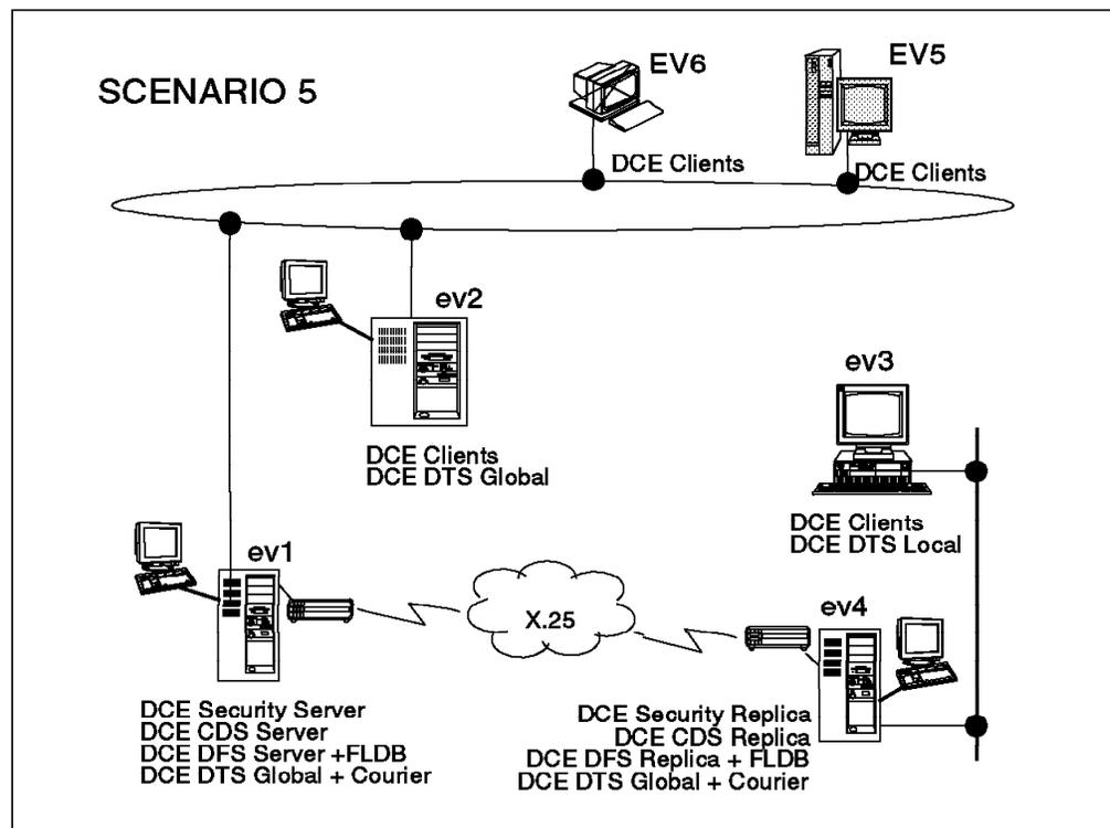
Figure 45. Scenario 5: A Large Branch Connected via X.25
