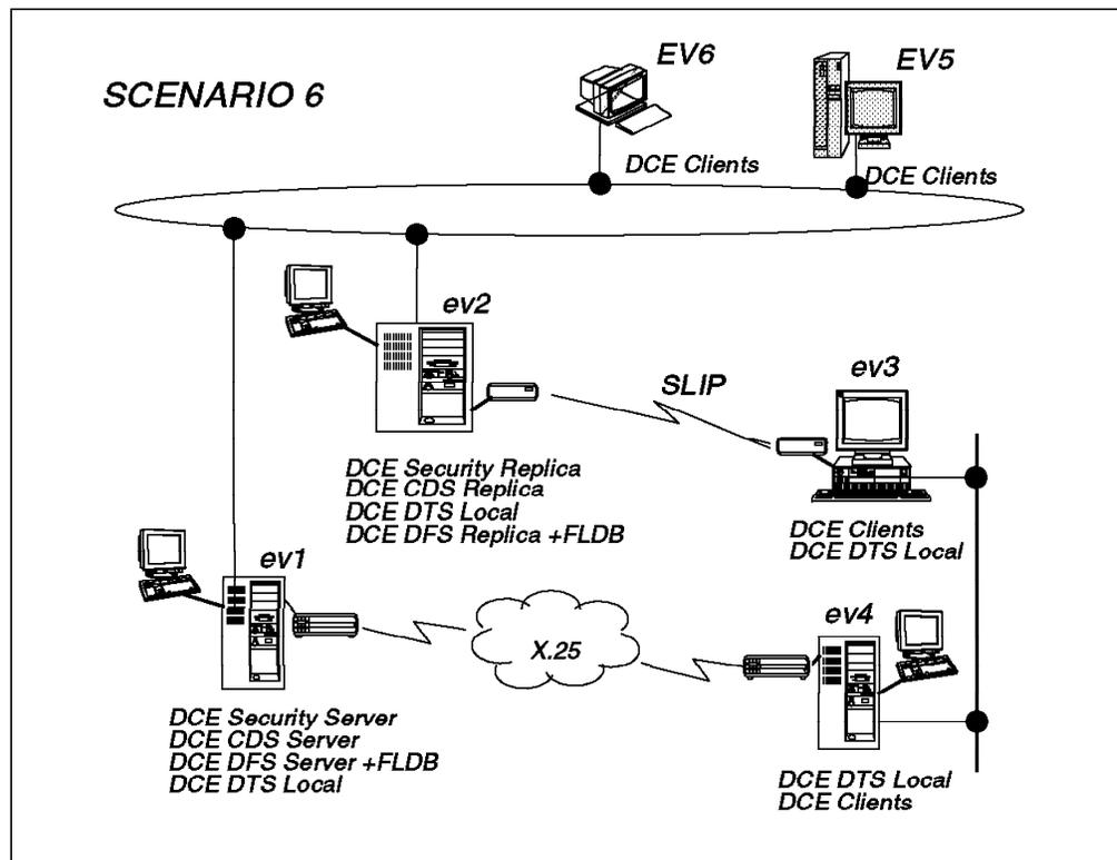
Figure 46. Scenario 6: A Branch Connected with Two Links
