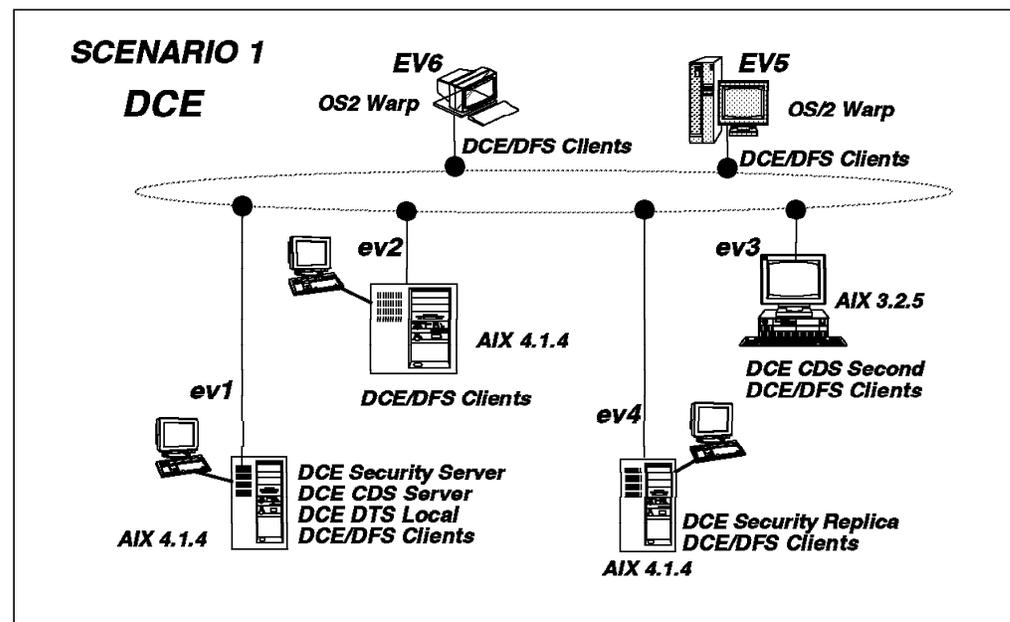
Figure 11. Cell with DCE Components and Related Platforms
