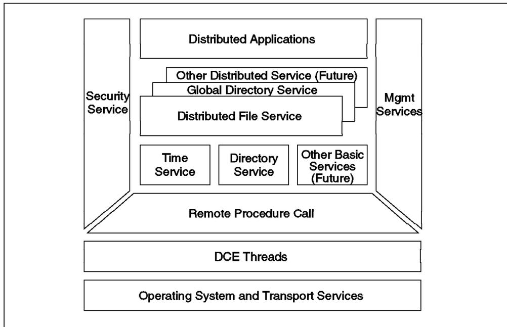
Figure 6. DCE Architecture
