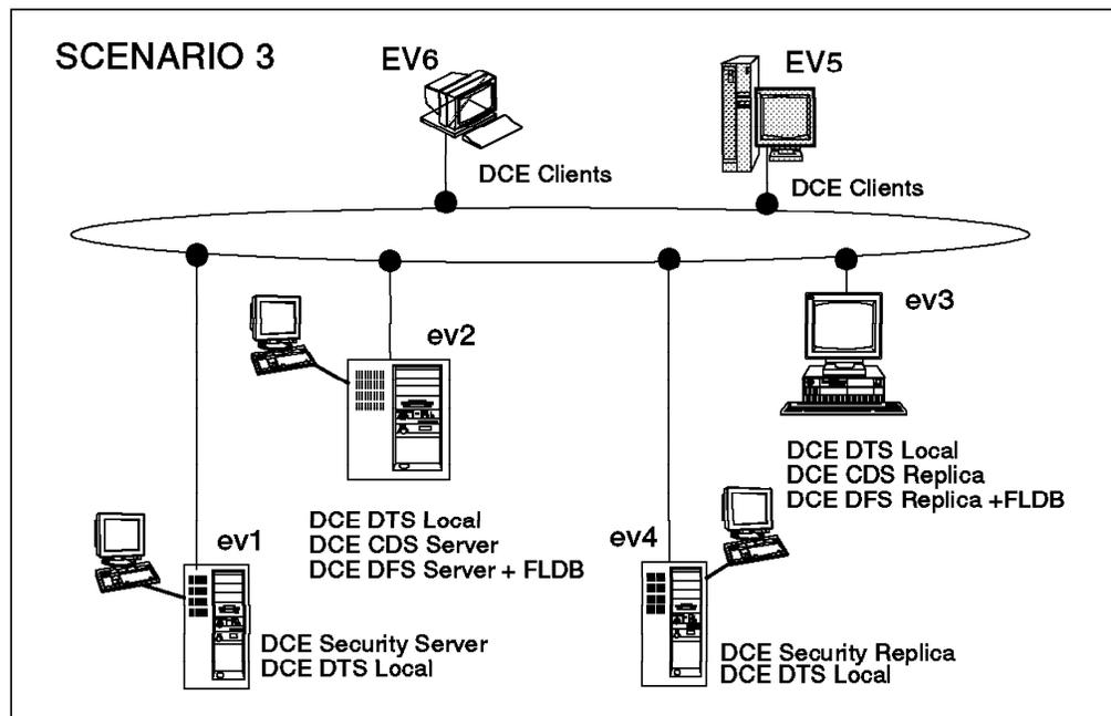
Figure 43. Scenario 3: DCE Servers on Different Machines
